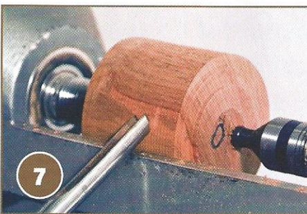
7 With the lathe set at a low speed to counteract the out of balance effect, start to shape the first side of the box
