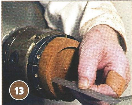
13 Check that the side of the recess is square by lining up a steel rule with the bed of the lathe
