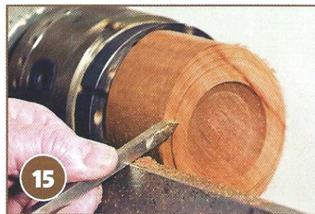
15 Now mount the base in the chuck and remove some of the inside before starting the spigot for the lid. Complete the turning of the spigot to a size that will give a jam fit for the lid
