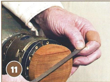
11 With the lid held in the chuck, clean up the face. To achieve the desired shape it is essential that the face of the lid is perfectly flat
