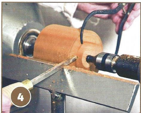
4 When the blank is at the required size, cut a spigot on each end to suit the size of the jaw chucks. On each end cut a second spigot of 80mm (3 1/8in) diameter by about half a millimetre thick to provide a datum for when forming the elliptical shape
