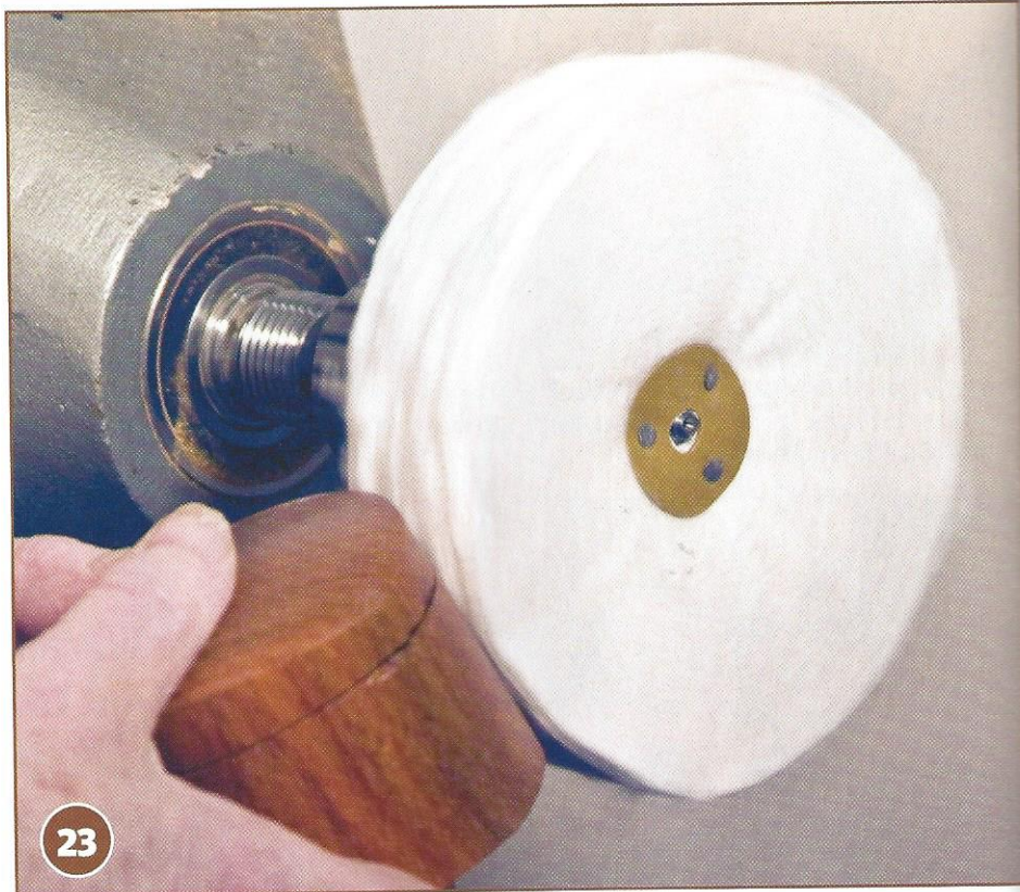
23 The final process is to polish the complete box on a buffing wheel loaded with a polishing wax
