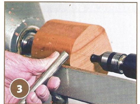
3 You are now ready to start turning the blank. The first few cuts made will remove the corners of the piece, and before long the piece will be round
