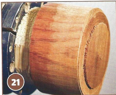
21 In order to finish the bottom, use a piece of scrap wood to make a jam chuck to hold the box
