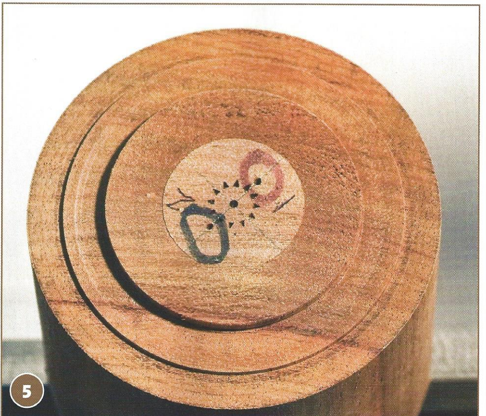
5 Mark centre points at the intersection of the diagonal and the circle on both ends and take care to ensure they correspond
