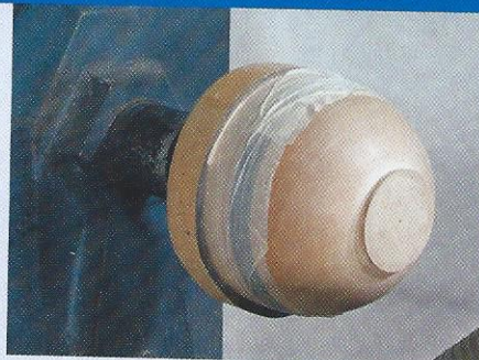
17 Fit your bowl on the jam chuck. If you lack confidence, tape it in place
