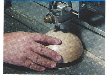
23 Run the bowl through the bandsaw avoiding fingers
