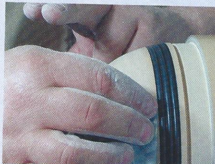
20 Sand. Remove the tape and take care to sand to the edge of the beads. Remove any dust. Apply sanding sealer
