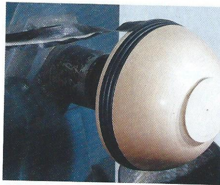
12 Once dry remove the tape carefully and remove from the lathe
