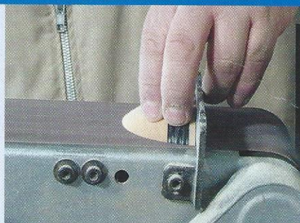
28 The small pieces can be placed against the fence while sanding
