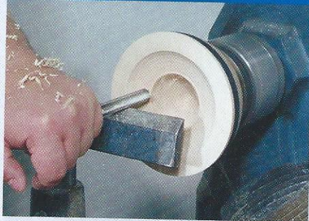
13 Mount your bowl in your chuck and remove the centre with a 10mm (3/8in) square grind bowl gouge. Try to achieve the best possible cut from your tool
