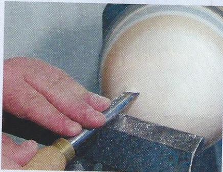
19 Use a 12mm (1/2in) round skew to shear scrape the outside to blend the two surfaces together
