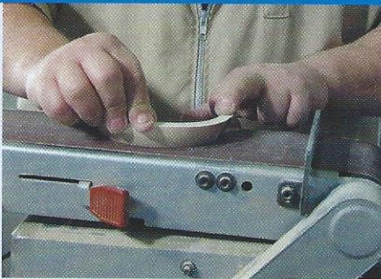
27 Using a belt sander sand the edges of the pieces evenly to ensure parallel sections. Repeat with all pieces
