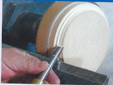
16 Mount a scrap blank on the lathe and turn a spigot to fit the inside of your bowl
