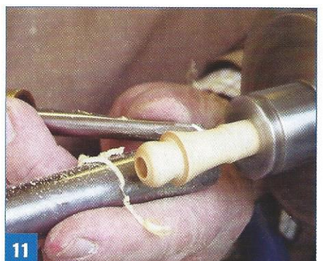
11 I shaped the hat using the point tool again. Note the position of my left hand on the tool rest
