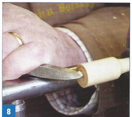
8 I found the centre of an 18mm ( \frac{23}{32} in) cylinder using an Eli Avisera \frac{3}{6} th Bedan
