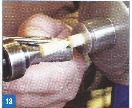
13 From a 10mm (3/8in) cylinder, I turned an arm, again with my ubiquitous point tool. Repeat this process for the second arm and sand and polish
