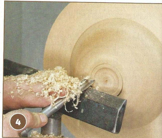
4 Refine the spigot and outside bowl shape with a 12mm (1/2in) round skew chisel
