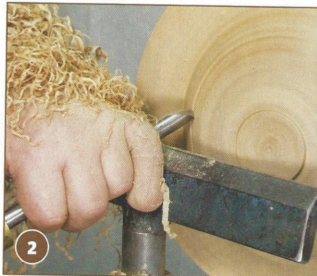
2 When approaching the final shape, re-sharpen the tool so you are able to produce the best possible cut straight from the tool
